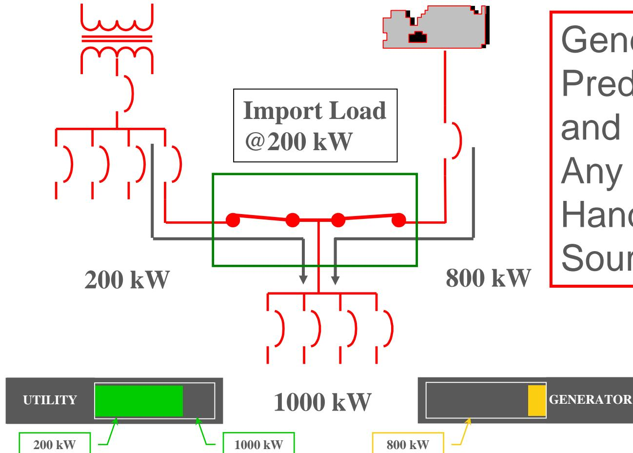
Generator is Ramped to a Predetermined kW Value and Holds. Any Load Variations are Handled by the Generator Source
