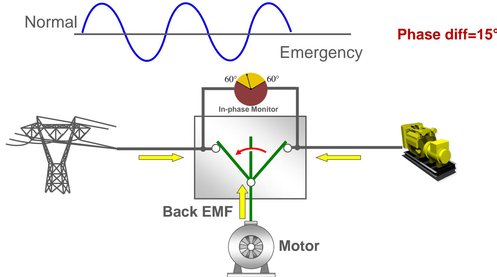
The inrush current is limited < 6 time running current of motor by the function of *In-phase Monitor*
