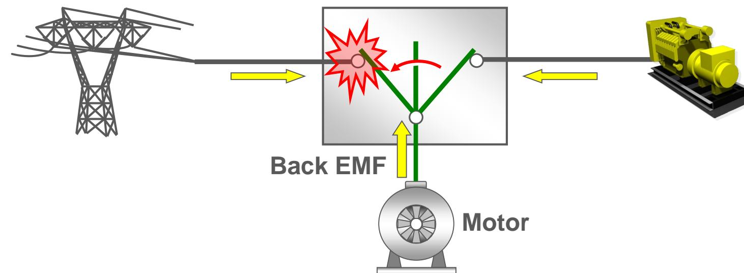
The inrush current can go up to max 18 time the running current of motor cause the CB trip
