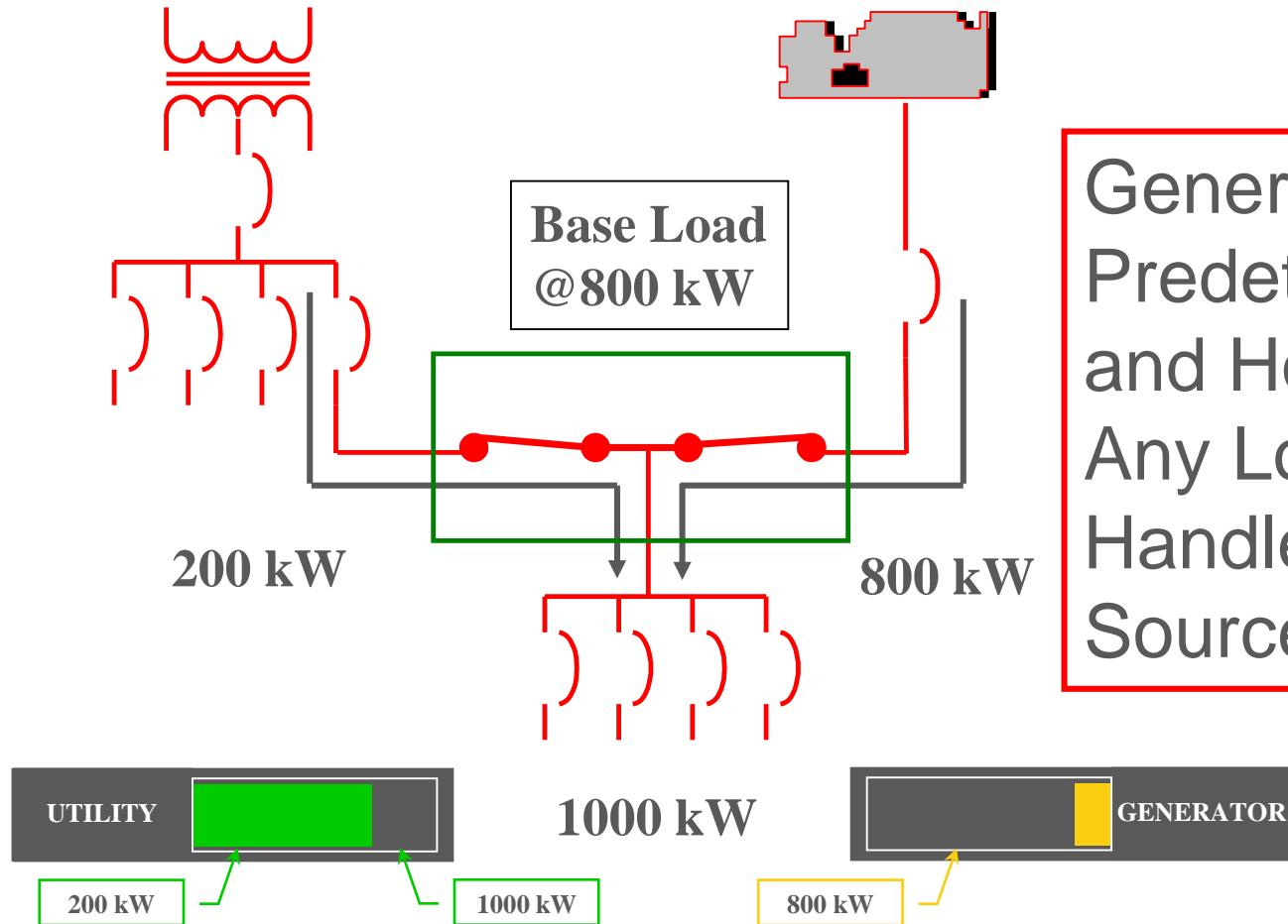
Generator is Ramped to a Predetermined kW Value and Holds. Any Load Variations are Handled by the Utility Source
