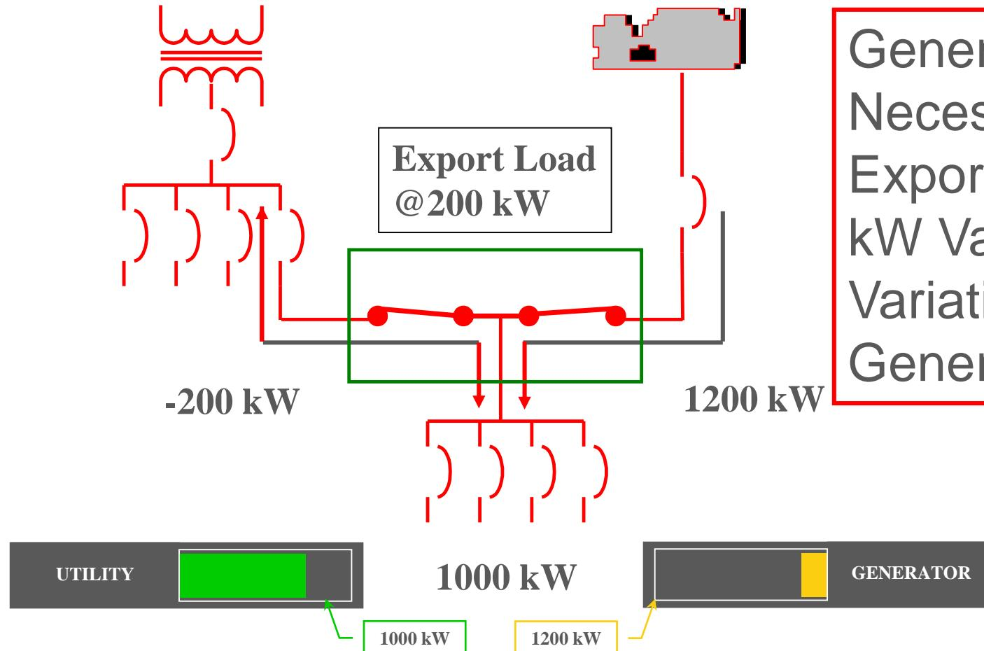
Generator Produces the Necessary Power to Export a Predetermined kW Value. Any Load Variation Are Handled by Generator Source.
